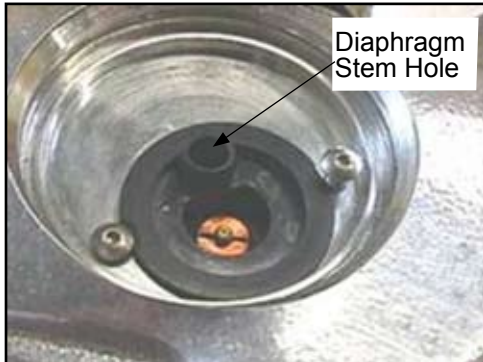
Figure 5: Button Screws Installed.
