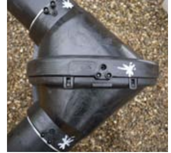
Completed Gemini Elbow.
